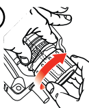
Firmly maintain the chuck and tighten the drill bit using the knob until it stops moving You are ready to sharpen
