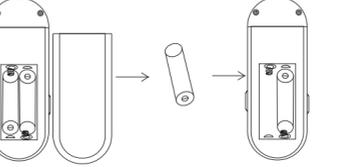
**2) Press and hold the "Arm" button while inserting the battery again. The control panel will emit 10 long beeps followed by 5 short confirmation beeps.**
