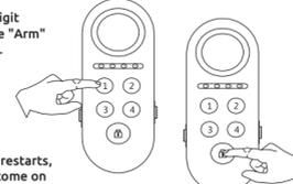
**3) Enter the new 4-digit code and press the "Arm" button to confirm.**
