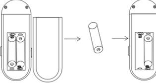
**2) Press and hold the "1" button while inserting the battery again. Press and hold the button until the control panel emits 6 long beeps and 2 short beeps.**
